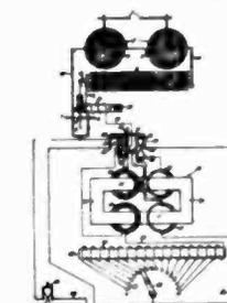
1. A high frequency discharge apparatus comprising a discharge circuit, a charging circuit, a supply circuit, an induction apparatus having a plurality of windings, means for connecting one of said windings to the supply circuit and the other of said windings to the charging circuit, and means for connecting both of said windings to the charging circuit.
