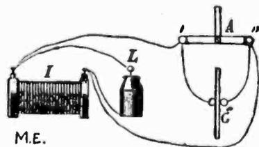
The experimenter must be careful when carrying a charged Leyden jar not to touch the brass ball (connecting with the inner coating) with the free hand, as a tremendous shock will be the consequence and in most cases the jar will be dropped and of course broken
