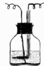
If the two outleading wires are now connected to an old, nearly worn-out dry cell, the thin capillary thread of mercury in the fine point changes its position. The thread will move a greater distance the stronger the current is. Too high a voltage squirts the mercury out through the fine aperture. Too much mercury in the tube has the same effect.
