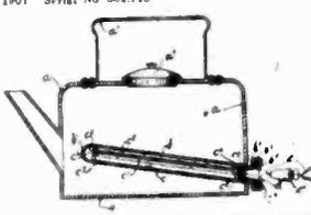
1. In combination with a kettle, a shallow rectangular chamber therein having one end open and extending outside the kettle, said chamber being inclined in relation to the kettle, a frame removably held in said chamber and electric heating coils on said frame.
