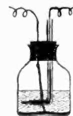
If the two outleading wires are now connected to an old, nearly worn-out dry cell, the thin capillary thread of mercury in the fine point changes its position. The thread will move a greater distance the stronger the current is. Too high a voltage squirts the mercury out through the fine aperture. Too much mercury in the tube has the same effect.
