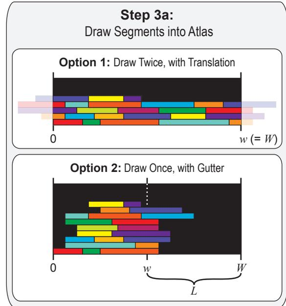
Fig. 8. *Segment atlas wrapping*. Because current generation GPUs do not support arbitrarily long 1D textures, the segment atlas must be wrapped to fit in a 2D texture. One option is to draw the atlas twice, wrapping segments that fall outside the width  $w$  (shown faded). Another option is to establish a gutter of size  $L$  to catch segments that fall outside  $w$ . Here  $W$  is the maximum texture width, and  $L$  is the maximum segment length.
