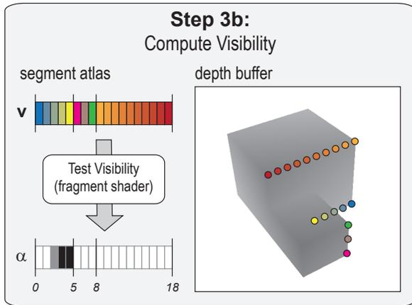
Fig. 9. *Visibility Testing*. The first three segments of Figure 7 are shown. Each sample in the segment atlas corresponds to a fragment. The fragment shader uses the screen space position  $v_j$  to test the sample against the depth buffer, recording the result in the visibility value  $\alpha_j$ . Colors are the same as Figure 7.
