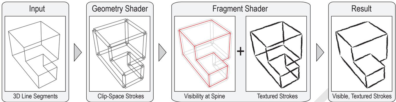
Fig. 3. *Steps in the spine test method.* The input is a set of 3D line segments. A geometry shader projects the line segments and creates clip-space strokes, preserving the homogenous positions for perspective-correct interpolation. A fragment shader checks visibility at the spine of the stroke, and computes a texture color. The visibility and texture are combined to produce the final result.
